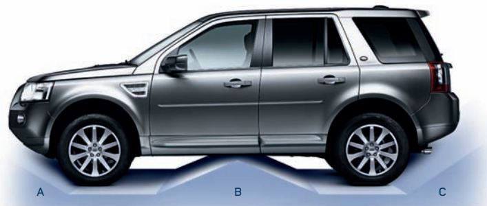
Off-road Geometry A B C Approach Angle 31° Ramp Break Over Angle 23° Departure Angle 34°
